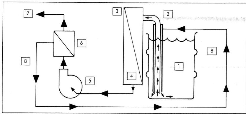
Oily wastewater [1] is drawn from the drum\* into the pickup tube [2] and fed to the prefilter assembly [3] for removal of solid particles which are collected in the cartridge filter [4]. From there, the smooth permanently lubricated pump [5] transports the wastewater under pressure to the membrane [6].
